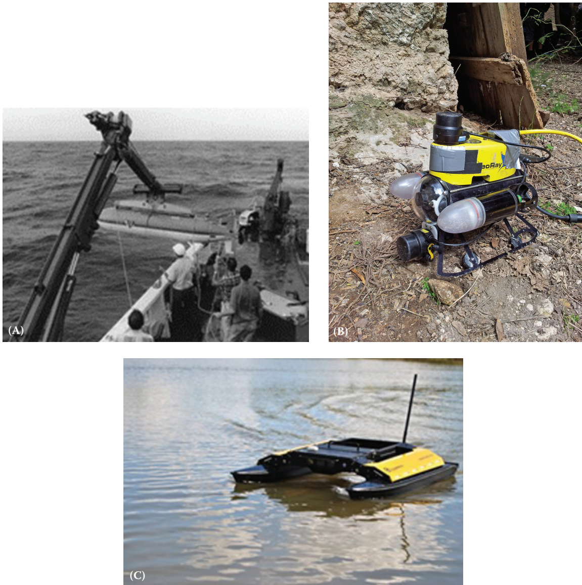
Figure 6.1 Examples of underwater robots: (A) Deployment of SPURV, the first autonomous underwater vehicle (AUV) (photograph courtesy of the Applied Physics Laboratory, University of Washington, Seattle). (B) A VideoRay underwater remotely operated vehicle (ROV). (C) This robot is a ClearPath Robotics Kingfisher ASV.
