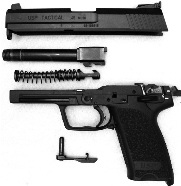
Figure 1.10 The Heckler & Koch USP Tactical pistol chambered in .45 ACP. The USP is recoil operated, using a modified Browning action. Note the differences between this recoil action, swinging link, and blowback designs compared with Figure 1.9. (Image from author's collection.)
