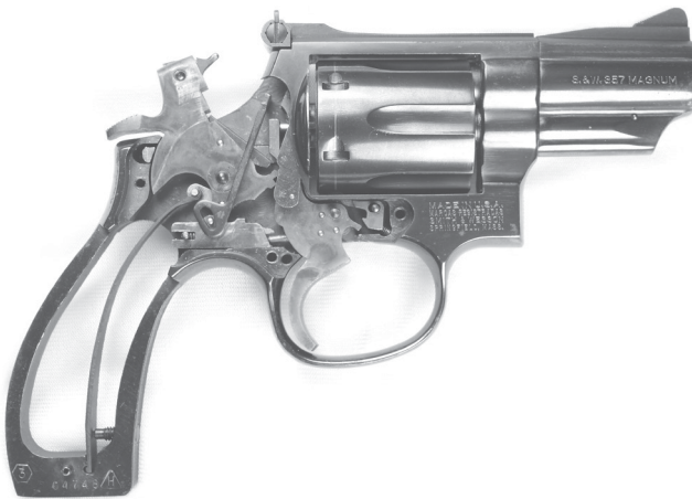
Figure 1.6 A Smith & Wesson Model 19 in single action firing condition, note the movement of the mainspring as compared with its position in Figure 1.5. The side plate has also been removed, revealing the hammer block safety and the linkage between the hammer and trigger. (Image from author’s collection.)
