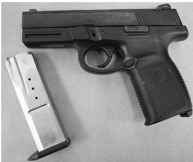
Figure 1.12 The Smith & Wesson Sigma SW40E and magazine. The Sigma series were the first polymer-framed pistols from Smith & Wesson. The trigger press had a more traditional double-action feel: long and smooth. Smith & Wesson chose to use steel-bodied magazines instead of polymer. (Image from author's collection.)
