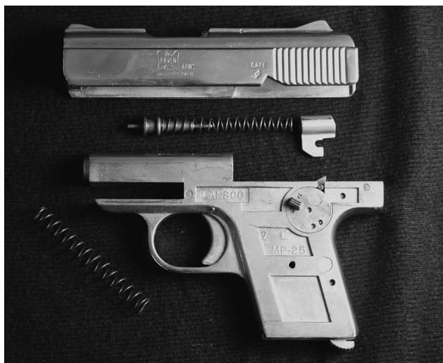
Figure 1.11 The Raven Arms MP-25, chambered in .25 ACP, is a striker-fired blowback pistol. The striker spring is cocked when the slide is retracted. The other spring is the recoil spring, which sits in the shroud surrounding the barrel. (Image from author's collection.)
