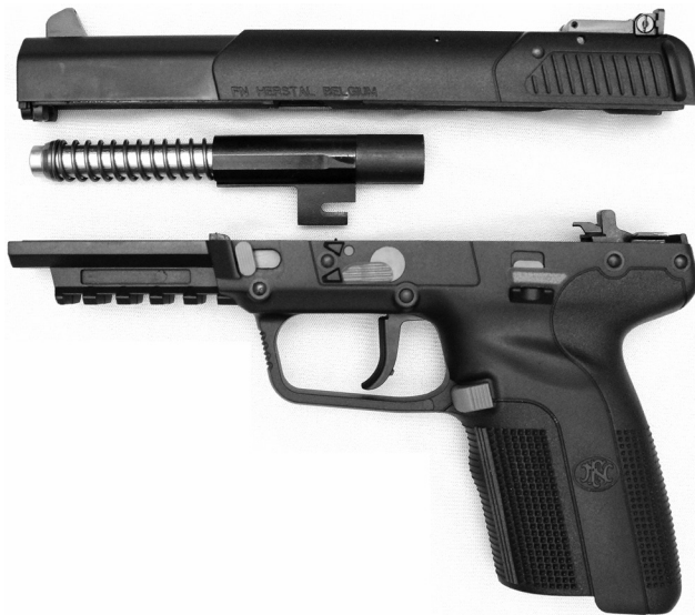
Figure 1.8 The FN Five-seveN is a delayed blowback pistol. Although there is no externally visible hammer, this is not a hammerless design. The hammer is seen at the rear of the frame, next to the ejector, which has a hooked appearance. (Image from author's collection.)
