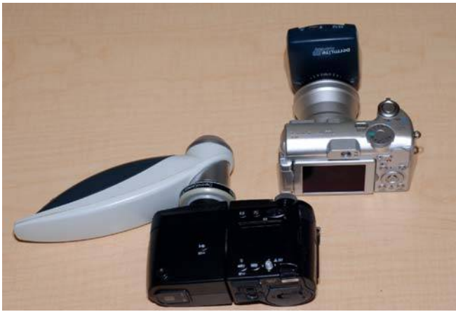
Figure 2.14 Most handheld dermoscopes can be coupled to a camera via an adapter. In this image the handheld DermoGenius is attached to a Nikon camera and the handheld DermLite is attached to a Canon camera.
