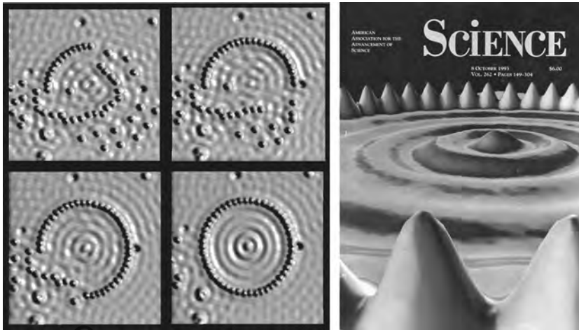
FIGURE 1.5 IBM’s Quantum Corral. In 1993, a ring of 48 iron atoms was arranged one at a time (four steps are shown) on a copper surface using the tip of a low-temperature STM. (We will learn more about the STM in Chapters 5 and 6.) The STM was then used to capture an image of the ring, which measures about 14.3 nm across. The iron atoms confine some of the copper’s surface electrons, and this barrier forces the electrons into quantum states, visible as concentric standing waves inside the corral. A three-dimensional rendering of this astounding achievement appeared on the cover of Science . (Corral image originally created by IBM Corporation. Journal cover from Science Vol. 262, No. 5131, October 8, 1993. Reprinted with permission from AAAS.)
