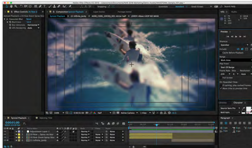
Figure 1: This screenshot of After Effects CC 2015 highlights the timeline interface element (bottom), where layers 2 and 3 are media sources with content that has been trimmed (the dark yellow regions to the right of the relatively brighter yellow), but is still accessible if needed (Adobe).
