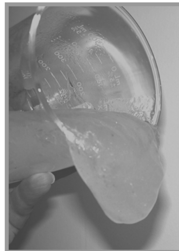
FIGURE 9.5 Example of a complex cross-linked gel.
