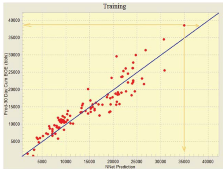
FIGURE 2.10 Cross plot of observed (measured) output versus neural network prediction for the training dataset. The largest field measurement is 3850 bbls.
