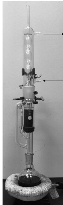
FIGURE 2.19 Asphaltene separation by Soxhlet extraction. (Courtesy of Vargas Research Laboratory, Rice University, Houston, Texas.)
