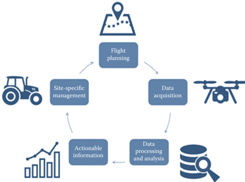
FIGURE 6.2 Life cycle of a sample PA application with UAS as a support tool.
