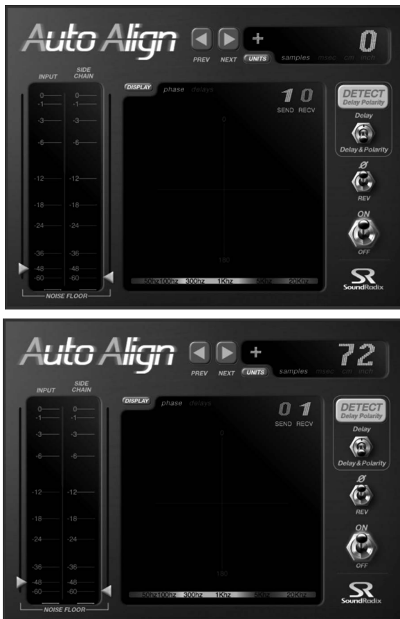
Figure 4.18 Auto Align , two signals compared and phase-aligned (72 sample delay between them).
